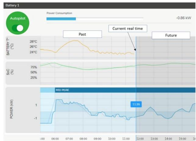
Figure 4 Example of real-time battery monitoring in the EMS.
