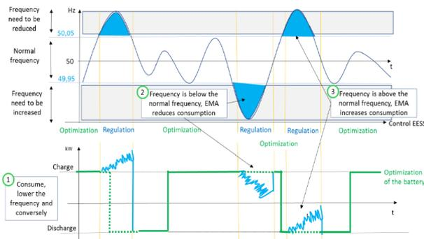
Figure 5 Frequency regulation using BESS.
