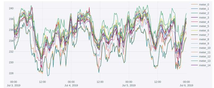
Fig. 2: Example of voltage profiles for 15 meters during three days, showing the strong similarities between data
