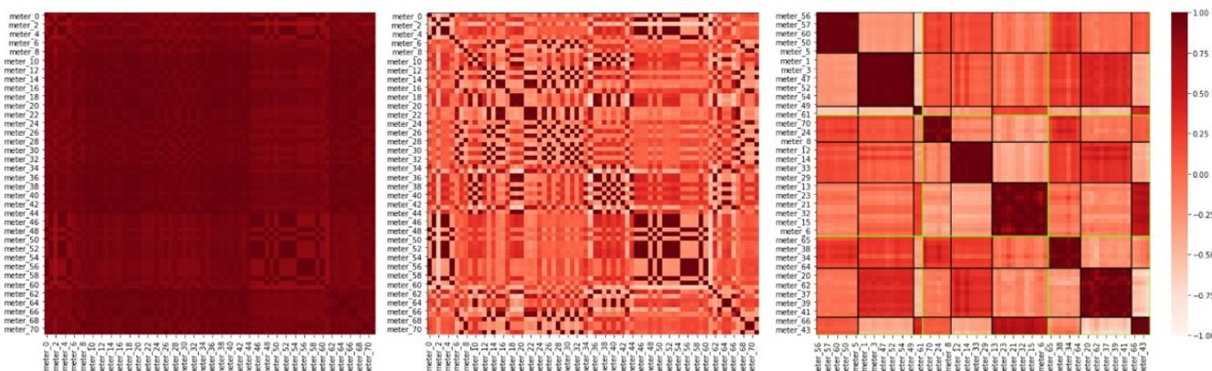
Fig. 3 Correlation matrices between raw voltage profiles (left), processed voltage profiles (center) and the same processed voltage profiles after the meters have been rearranged by feeder and phase (right), where green lines delimit the different feeders, and black lines delimit the three phases. Correlation ranges from -1 (white) to 1 (red).
