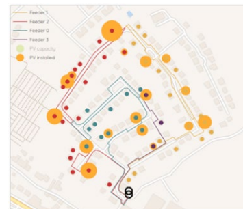
Fig. 2: Location of installed PV productions – initial state
