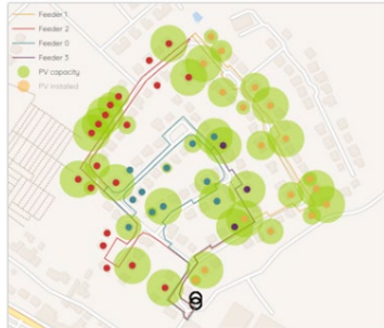
Fig. 8 Network hosting capacity for PV – balanced network
